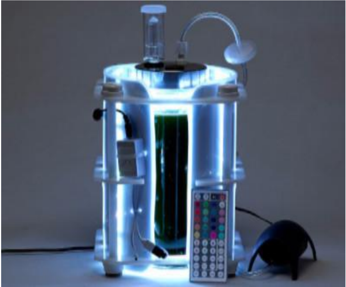
Figure 14: UTEX RGB-Led lighting platform (The University of Texas at Austin)
